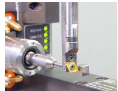
Extremely fast measurement of non-rotating tools
