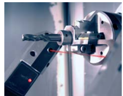
Fast detection of micro-wear at the cutting edge
