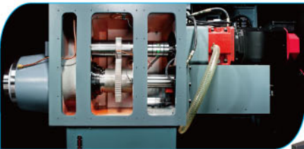
FANUC A15 / 7000 with GERMAN ZF gear box 1:8 gear ratio
