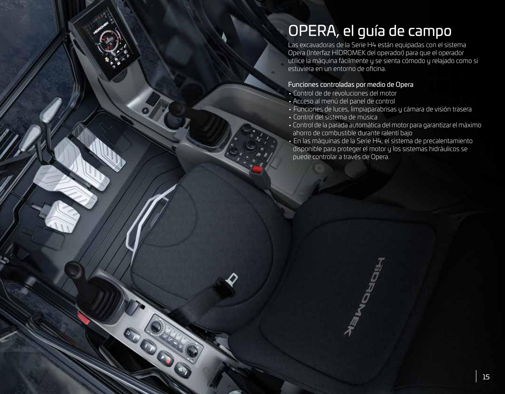
The image shows the operator's cab of an excavator. The central focus is the OPERA control system, which includes a large digital display at the top left showing engine RPM and other metrics. Below the display are various control levers, buttons, and a gear shifter. The operator's seat is visible, featuring the 'HIDROMEK' logo. The overall design is modern and ergonomic, aimed at providing a comfortable and efficient operating environment.
