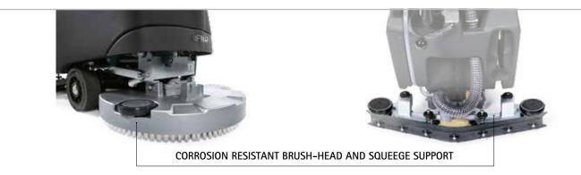
The brush-head and the squeegee support are completely made in aluminum, that makes them robust and shock proof. Besides, they are properly treated to be corrosion resistant: in this way MMx50 B/Bt can be used even in environments such as swimming pools or dairy factories offering high performances and productivity.
