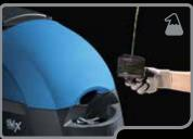
The measuring cap of the tank allows to pour the proper detergent quantity, avoiding wastes or excessive use
