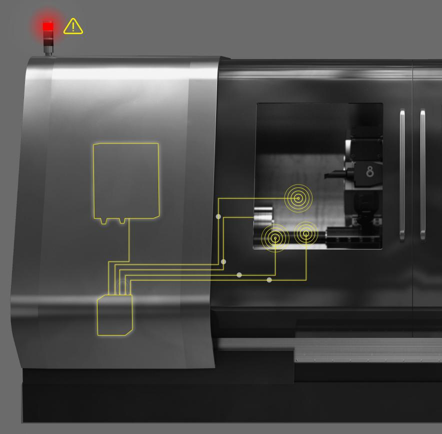
Collision detection will monitor the machining force or vibration and instantly stop machining in case of an overload.
