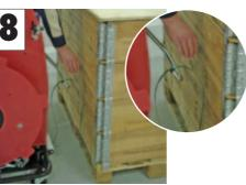
The automatic strap-lifter brings the end of the strap to working height without the operator needing to bend.
