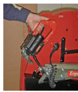
For pallets with a height below 70 cm the locking tool can be detached and placed on the package.
