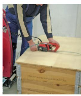
The strap will then be tensioned and sealed on the top of the pallet.
