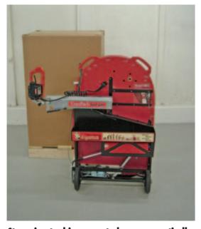
Strapping tool is supported on pneumatically operated tool lift achieving the effortless application to strap.
