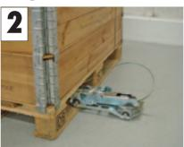
The patented ChainLance guides the strap through the pallet void ...
