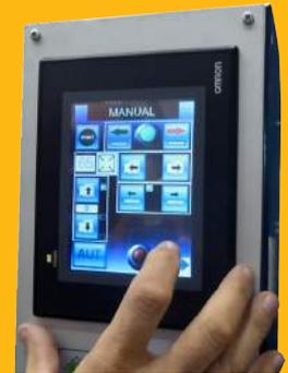
It allows you to select between the different stored strapping programs with pressing a button.
