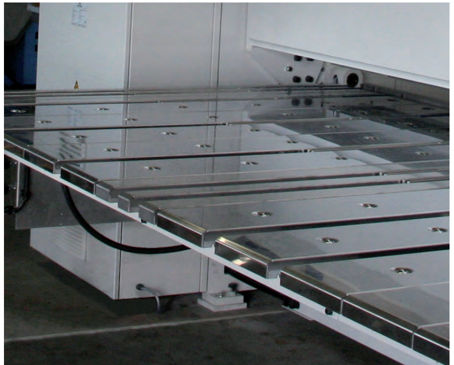
Gauge table, 1,600 mm, closed, with ball transfers
