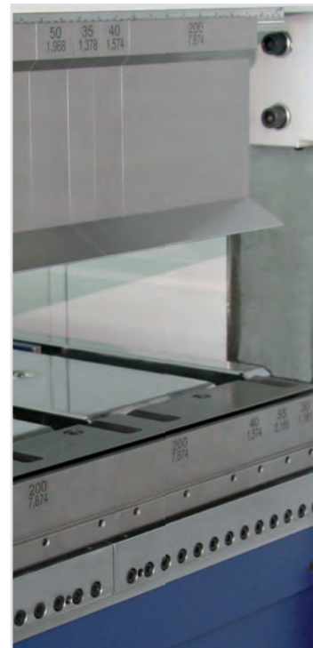
The motor-driven lowerable folding beam and the motorized folding centre adjustment are included in the standard version.
