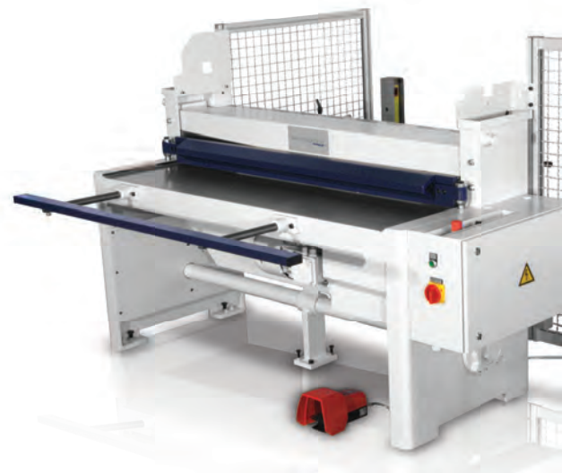
Standard: MSHU with rear guarding via 2-beam light barrier incl. side protection grid
