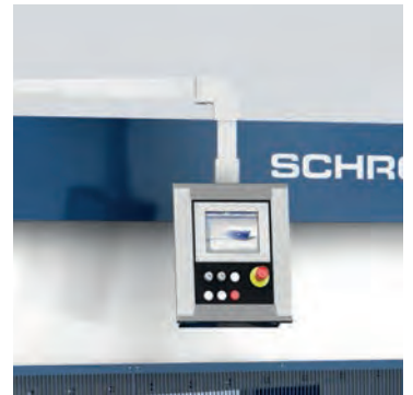
Option: touchscreen control CGS 80 on swivel arm
