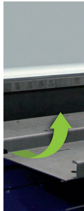
Up-and-Down-function: counter folds without turning upside down the sheet
