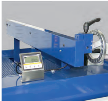
Manual back gauge, adjustable from the front, with digital readout
