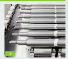
Patented reversible leveling rollers
