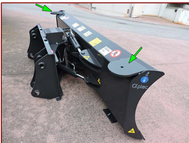
▲ Placas soporte para receptor laser - opción Support plates laser receiver - option
