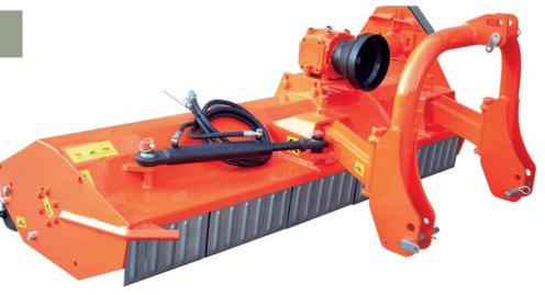
The universal TLGJ flail mower is a machine used for shredding grass and pruning of vineyards and orchards. The mechanical or hydraulic transversal displacement (max 40 cm) allows the employment in decentralized position, to approach to plantings, to orchards, etc. The machine is provided with a connecting plug with three points, reason why it can be used with any kind of tractor, both caterpillars and farm tractor.
