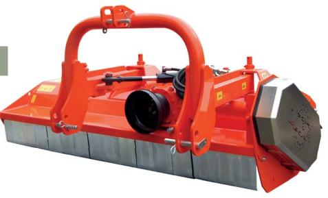
The universal TLC-S flail mower is a machine used for shredding grass and prun-ing of vineyards and orchards. The mechanical or hydraulic transversal displace-ment (max 40 cm) allows the employment both in normal and in decentralized position, to approach to plantings, to orchards, etc. The machine is provided with a connecting plug with three points, a rear opening cover that facilitates the inspec-tion. It can be used with any kind of tractor, both caterpillars and farm tractor.
