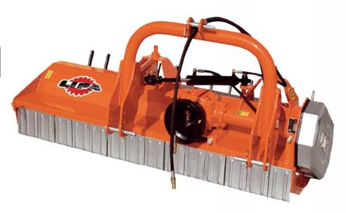
The universal TLS flail mower is a machine used for shredding grass and pruning of vineyards and orchards. The mechanical or hydraulic transversal displacement (max 40 cm) allows the employment in decentralized position, to approach to plantings, to orchards, etc. The machine is provided with a connecting plug with three points, reason why it can be used with any kind of tractor, both caterpillars and farm tractor.
