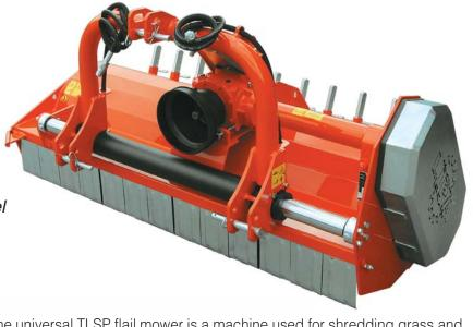
The universal TLSP flail mower is a machine used for shredding grass and pruning of vineyards and orchards. The hydraulic displacement (max 40 cm) allows the employment in decentralized position, to approach to plantings, to orchards, etc. The machine is provided with a connecting plug with three points, reason why it can be used with any kind of tractor, both caterpillars and farm tractor.
