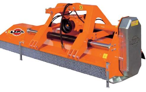
The universal TLR-P shredder is an ideal tool for the works in forestry, on grazing grounds and large areas. The machine is equipped with laterally adjustable anterior and rear connecting plugs, its reversibility allows you to overwork in the best way its performances and to choose the kind of working according to your requirements.
