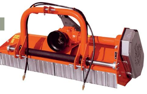
The universal TLGS shredder is a machine used for crushing grass and pruning of vineyards and orchards. The hydraulic displacement (max 40 cm) allows the employment in decentralized position, to approach to plantings, to orchards, etc. The machine is provided with a connecting plug with three points, reason why it can be used with any kind of tractor, both caterpillars and farm tractor.
