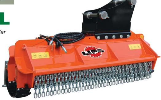
The hydraulic forest TLE-FL shredding head is perfect for crushing grass, canes and shrubs generally up to 10 cm of diameter, located near ditches, banks, uncul-tivated and wooded areas and all sorts of very steep lands. It can be applied to excavators weighing from 12 to 18 tons.
