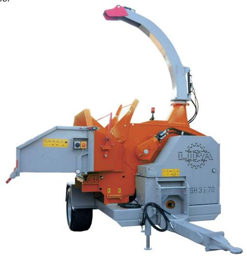
The M.T.L. 35.70 chipper is a machinery used for the production of calibrated and uniform chipped through the trituration of branches and trunks up to 35 cm of diameter. It is also used for the shredding of brushwood of every kind, even fibrous, like palm leaves. Driven by the PTO of the tractor, is ideal for agricultural and forestal companies and in particular for contractors dedicated to the promo-
