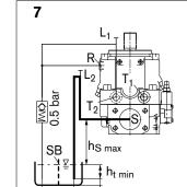
$h_{s max} = 800 \text{ mm}, h_{t min} = 200 \text{ mm}, h_{min} = 100 \text{ mm}, SB = Silencer plate (baffle plate)$
