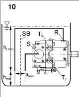
$\begin{aligned} &h_{\text{s max}} = 800 \text{ mm, } h_{\text{t min}} = 200 \text{ mm, } h_{\text{min}} = 100 \text{ mm,} \\ &SB = Silencer \text{ plate (baffle plate)} \end{aligned}$
