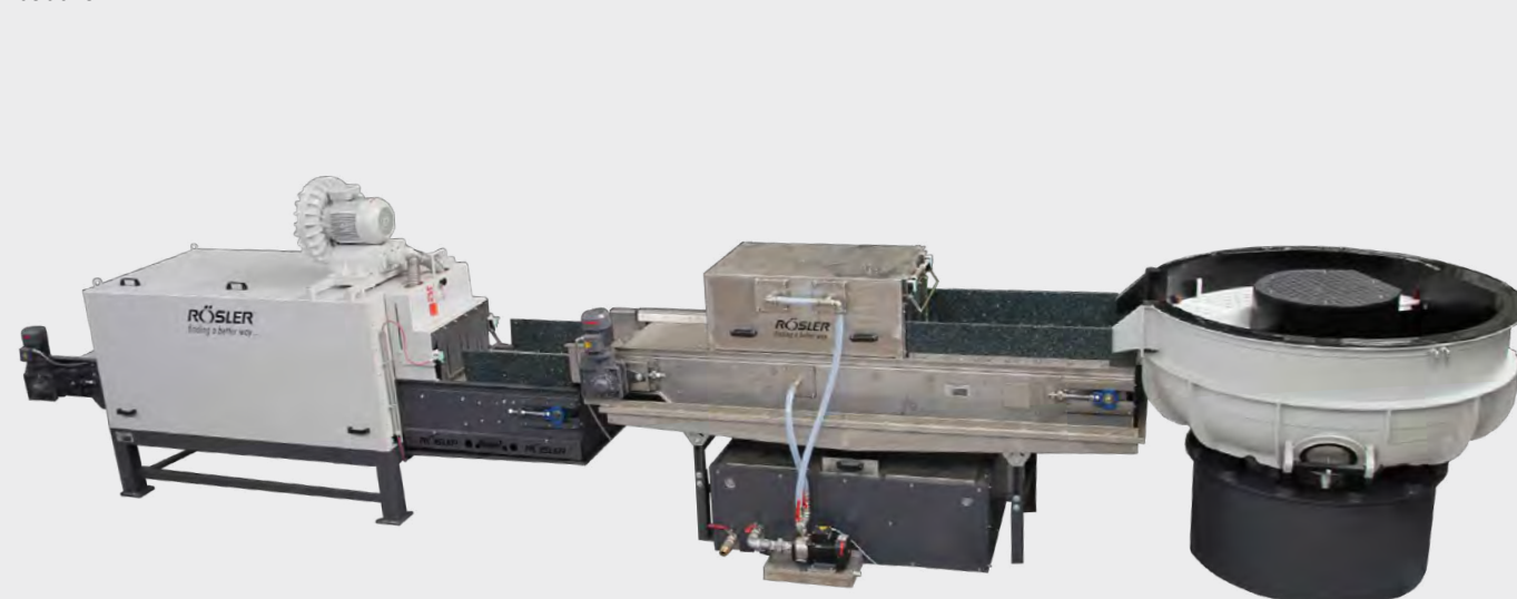
Rotary vibrator with belt spray washing station and hot air belt drier
