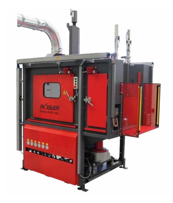
Satellite table blast machines are employed, whenever the work pieces are deemed critical or not allowed to touch each other during the process. The spectrum of applications ranges from delicate deburring to intensive shot peening. This machine type is particularly suitable for applications where only specific work piece areas require to be blasted. Turbine abrasive delivery technology as well as air blast systems can be installed.
