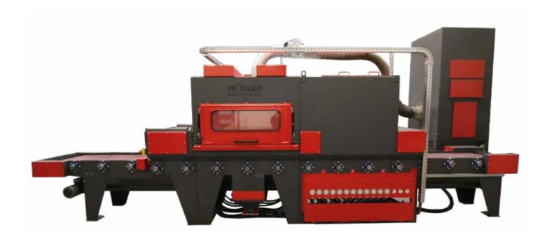
Continuous feed belt blast machines are used for cleaning, stripping and surface preparation prior to bonding or coating tasks in continuous feed operations. They are ideal for continuous manufacturing operations with relatively high work piece volumes. Practically no productive time is lost through work piece loading and unloading. The blast media is always thrown from above the belt. Oscillating movement of the blast nozzle(s) ensures optimum blast coverage.
