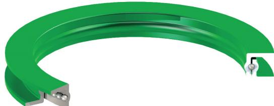
ISB agricultural slewing bearings feature a **flanged structure** and a single **full complement ball bearing without** spacers. They are supplied with surface **paint** that prevents corrosion, are **pre-greased, not toothed**, and not equipped with gaskets. They are able to support **very heavy axial loads** and turn at low speed.
