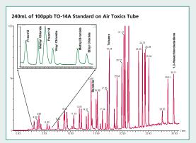
Sample analysis of an air toxics reference material demonstrating separation, detection, identification and quantification of a wide range of volatiles from freon through hexachlorobutadiene.
