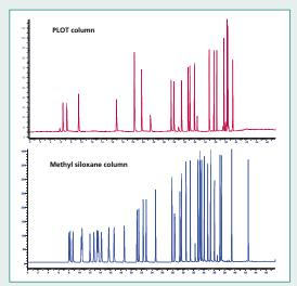
Demonstration of complete separation without sub-ambient oven temperatures, highly volatile analytes are fore-flushed onto a PLOT column, while less volatile analytes are separated on the methyl siloxane column. Each column is connected to its own detector so the two chromatograms are produced simultaneously.
