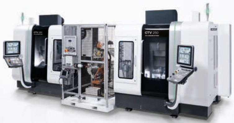
Manufacturing cell consisting of 2 x CTV 250 DF and one 6-axis robot for the fully automatic production of components for constant-velocity joints
