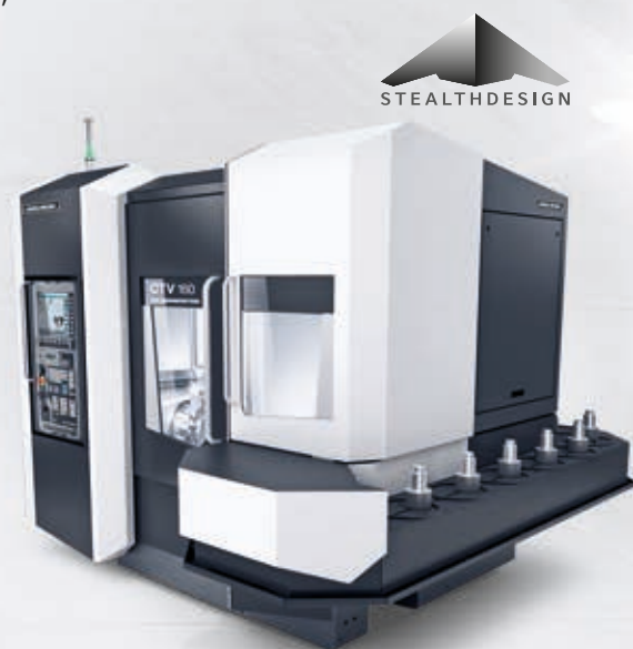
The CTV 160 has a footprint of just 10.7 m 2 including chip conveyor and automation
