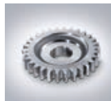
Automotive: Gear wheel manufactured on a CTV 160 // 42CrMo4 // 35 / 38 sec (OP10 / OP20)
