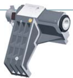
Main spindle up to ISM 127 PLUS (max. 6,000 rpm, or 59 kW and 4,000 Nm)
