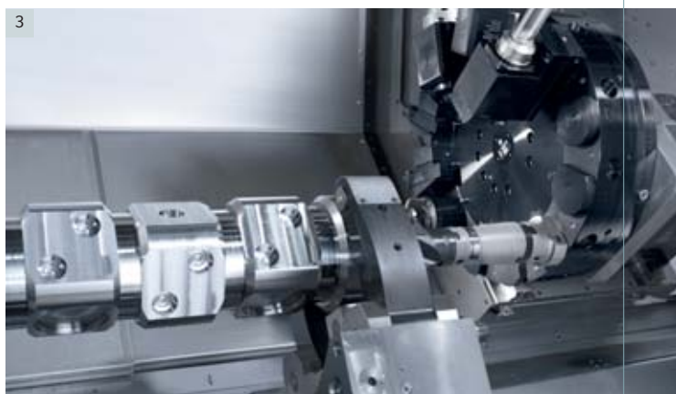
[1] Eccentric machining with the Y-axis on the counter spindle [2] Y-axis in the highly stable wedge slide design [3] Bezel with automatically traversable steady rest carrier for the vibration-free machining of long parts
