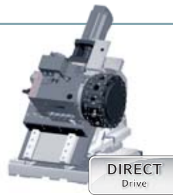
Star turret on the top right, also available as a Direct Drive (only for the beta 4A)
