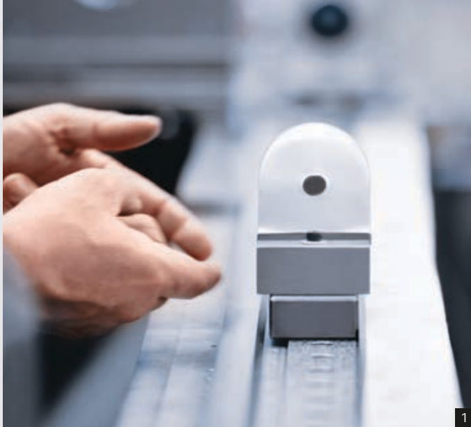
1: Multiple measurement of the guideways using an autocollimator 2: Scraped surface
