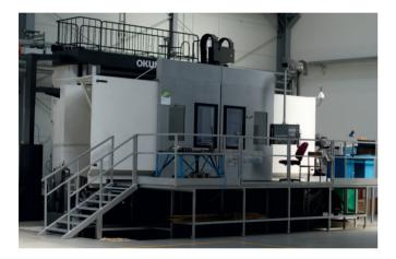
Our new machine Okuma VTR-350A has a double column turning centre which provides large capacity machining, with high rigidity and thermal stability for close tolerance machining. Suitable for machining workpieces with a max. turning diameter of Ø3500mm and max. length of 1600mm.
