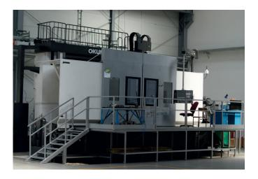
Our new machine **Okuma VTR-350A** has a double column turning centre which provides large capacity machining, with high rigidity and thermal stability for close tolerance machining. Suitable for machining workpieces with a max. turning diameter of **Ø3500mm** and max. length of **1600mm**.
