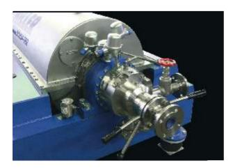
The centrifugal force generated by the rotation of the bowl rapidly settles the solids particles at the bowl wall, where they are moved towards the solids discharge ports by a screw conveyor.
