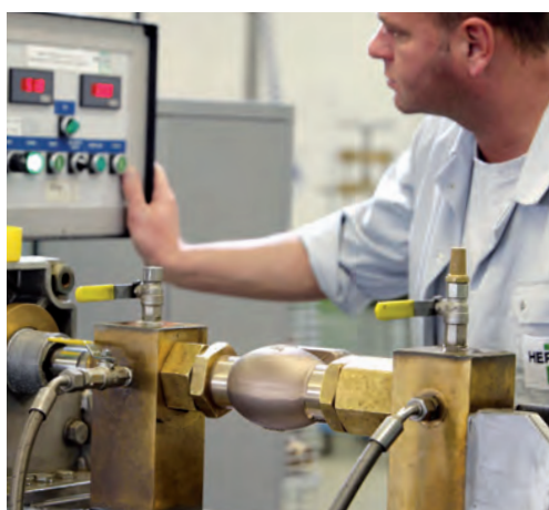
100 % tightness test of the valves at design pressure
