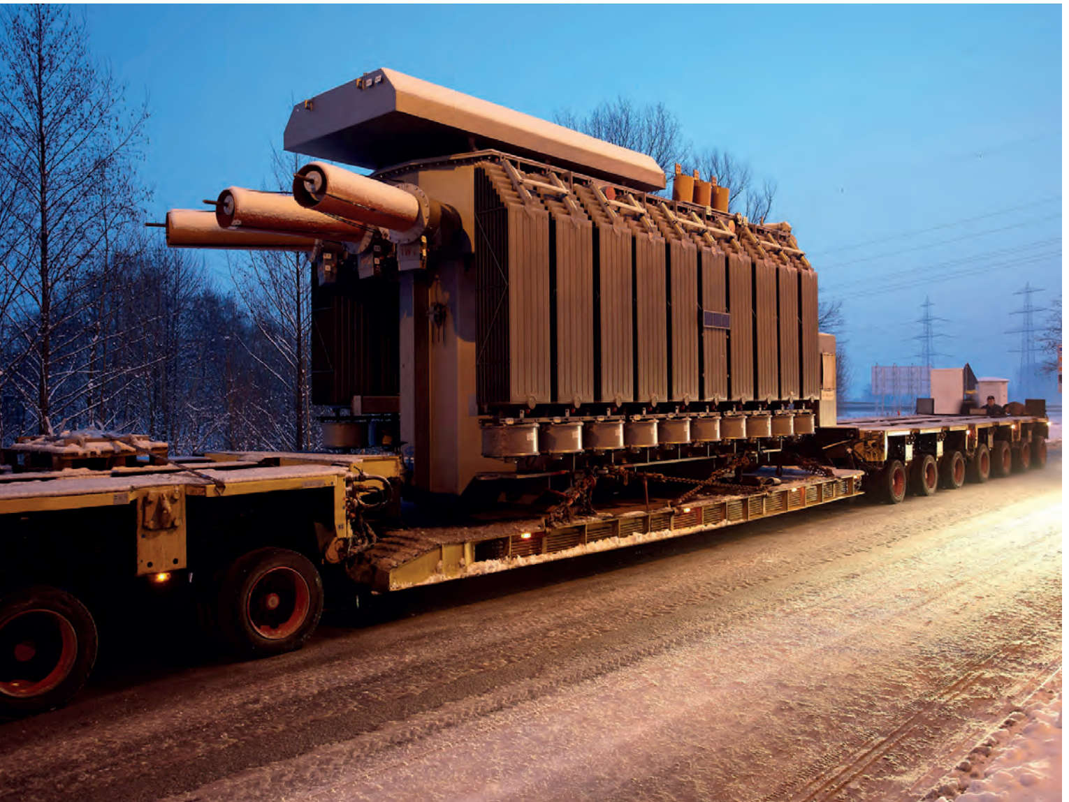
An oil-immersed transformer on its frozen way to the final place of installation. Equipped with HEROSE valves for low temperature applications.
