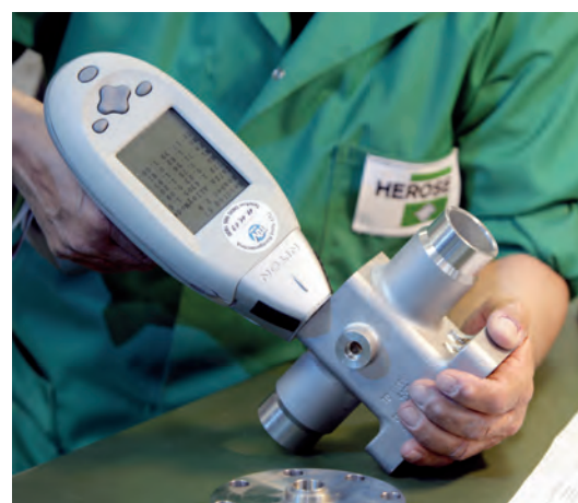
Material analysis and identification during the incoming goods check
