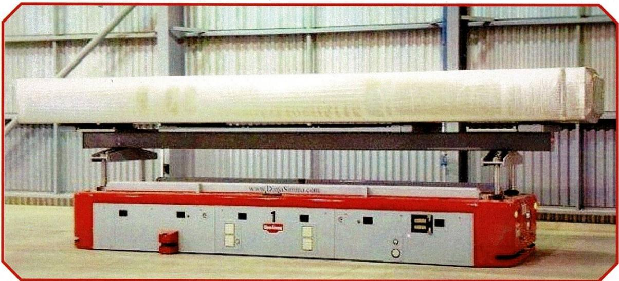
**AGV - WITH TOP LOAD PLATFORM TRANSPORT SYSTEM
