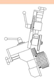
Infeeding device, showing the pressure rollers (adjusted manually) and the feeding rollers.
