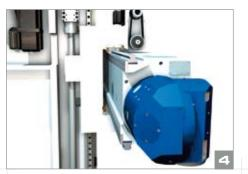
Close spacing of the guide tracks to the column and headstock results in short power transfer distances and thus higher rigidity for powerful milling and machining.
