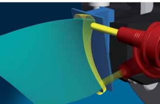
**Machining transition radii:** Regardless of the data quality, the entire blade can be machined very efficiently using ball mills.
