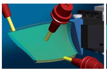
**5axis blade top milling:** Blade surfaces are finished in a continuous spiral toolpaths. The automatic lead angle correction ensures that endmills and bullnose endmills always cut with the front.
