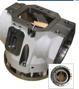
Machine: Unipro 5P with Siemens 840D Performance data: 100 kW (25.000 rpm HSK 63)
