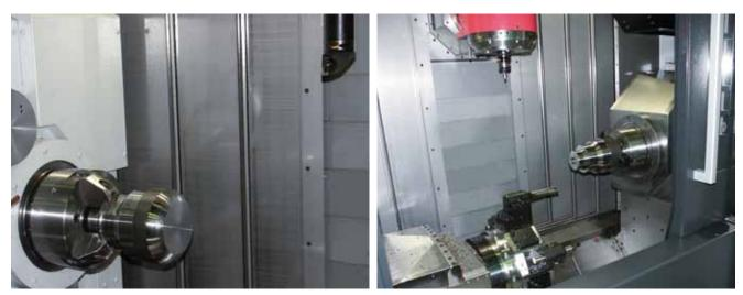
**Turning process.** Turning operations are programmed using the mill-turn module *mill*TURN. The module is seamlessly integrated into *hyper*MILL<sup>®</sup>: The turning process on the counter and main spindle was generated based on this.
