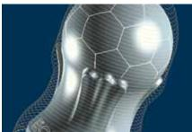
**5axis cavity cycles** The cavities package expands the 3D cycles to include simultaneous multi-axis machining. In comparison with the 3+2 strategy, it enables continuous machining and yields a better surface prevention feature that guarantees quality.
