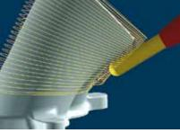
Undercut Machining: The 5Axis-cyc- Tube Milling: Complex and preciles allowing a complete machining of se tubes can be programmed and difficult-to-access undercut areas in a machined in one set up. The cycle continuous spiral movement. Thereby is designed to work on any surface high quality surfaces are achieved.
