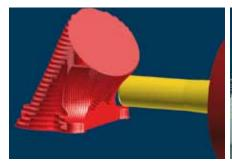
Roughing on any Stock: Arbitrary stock roughing can be based on an initial stock model or the remaining stock after any operation. Further, this approach works from any tool orientation.
