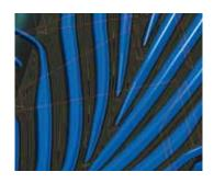
**5axis Top Milling** With pocket options generates a super fast finishing tool path normal to segment bottom.
