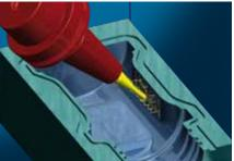
**5axis contour machining:** All that is nition of a reference contour. Engravings, contours and grooves do not need to be designed separately, thus eliminating time-consuming CAD programming of details.
