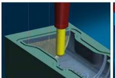
**Hub machining:** Milling paths can be calculated independently from the required for machining is the defitool position, which makes creating a program for every geometry a simple task. The tool positions are then taken into account in the 5axis rework cycle.
