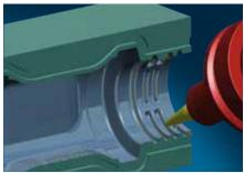
saxis halfpipe machining: Using this strategy from the Tube package, grooves can be easily programmed and milled by defining a reference curve, regardless of the profile or cross-section involved.
