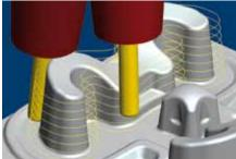
**5axis Swarf Cutting** The tool flank and wide path distances can be used to mill drafted faces without special tools. This reduces machine runtime and ensures premium quality single operation. Information on the surfaces.
