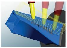
**5axis radial tangential machining:** This strategy helps to achieve smooth-finished surfaces with comparatively large stepdowns. Tool life is excellent: The highest level of dimensional accuracy can be guaranteed as the thermal growth of the spindle has no influence on peripheral milling.
