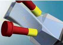
5axis rework: This converts 3D programs to 5axis simultaneous programs. *hyper*MILL<sup>®</sup> calculates collision-free tool paths, including the alteration of tilt angles. Rapid link tomated feature ensures that the tool movements are reliably optimised with 5axis technology.
