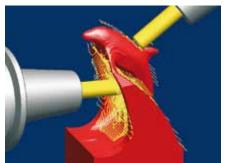
With undercut optimisation The "arbritrary stock roughing" strategy with undercut optimisation automatically recognises the areas which have collision-free tool paths, including already been machined with different the alteration of tilt angles. Fast tratilt angles. Redundant movements are avoided, tool paths are optimised optimised with 5axis technology. and machining times are reduced.
