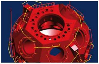
**5axis drilling** An automated function calculates the tool angles and takes into account all lead-in positions while also checking for collisions and optimising the path for 5axis processing.
