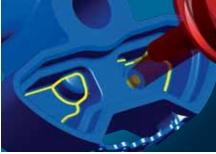
**5axis rest machining:** *hyper*MILL<sup>®</sup> combines fully automated machining with different fixed tool angles and 5axis simultaneous movements in a single operation. Information on the slope angle is not required for the operation.
