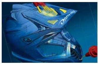
**5axis milling:** With the 5axis strategies from *hyper*MILL<sup>®</sup>, geometrically complex parts that up to now could not be milled or only with a great deal of manual effort can now be manufactured cost effectively. The fully automated collision avoidance ensures simple programming and a high level of process reliability.
