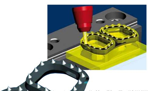
5AXIS swarf cutting: The larger depth-of-cut in 5AXIS swarf cutting reduce machining times and ensure a superior surface quality. Multiple axial and lateral infeeds also make this strategy suitable for roughing. Machining is optimised through the definition of milling and stop surfaces, and through stock tracking.
