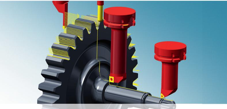
Mill turning. In one setup. No set-up changes.
