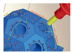
The 5axis drilling function is used to simply and automatically program drilling jobs with different tool angles in a single operation.
