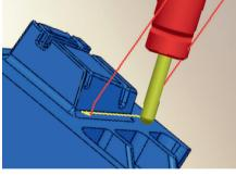
When using 5axis swarf cutting, the workpiece surface is machined with the tool flank. Large step-downs between paths reduce milling times.
