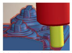
During stock roughing, stock tracking ensures active collision avoidance. The tool path is moved laterally in the case of a potential collision between the stock and the tool shank or holder.
