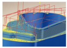
Z-level finishing and profile finishing can be combined for complete finishing jobs. As a result, machining can be automatically adapted to the requirements of individual model areas.
