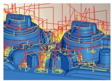
Referencing to previous rest machining allows areas that have not been machined to be cleared very quickly using a new tool and/or tool inclination.
