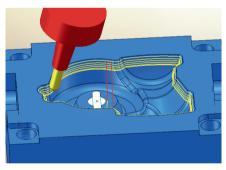
Steep areas can be machined plane by plane using 5axis Z-level finishing. Automatic collision avoidance ensures process reliability.
