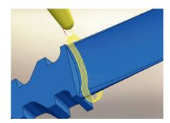
The Blade package offers optimised machining strategies for complete machining from top to bottom and the blade in the middle.
