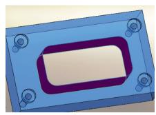
In addition to closed pockets, pockets with islands and pockets with open sides, *hyper*MILL® now also detects breakthroughs.
