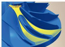
The automated functions in the Multi-Blade package minimise the number of process parameters that need to be defined.
