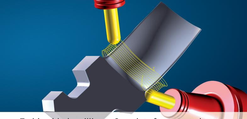
Turbine blade milling - Complete from top to bottom
