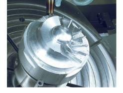
without the need of any second CAM product. Furthermore, multiblade cycles permit the use of conical tools, barrel, bullnose etc.
