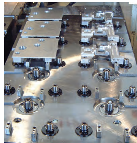
Clamping and locating mill parts on two bores.
