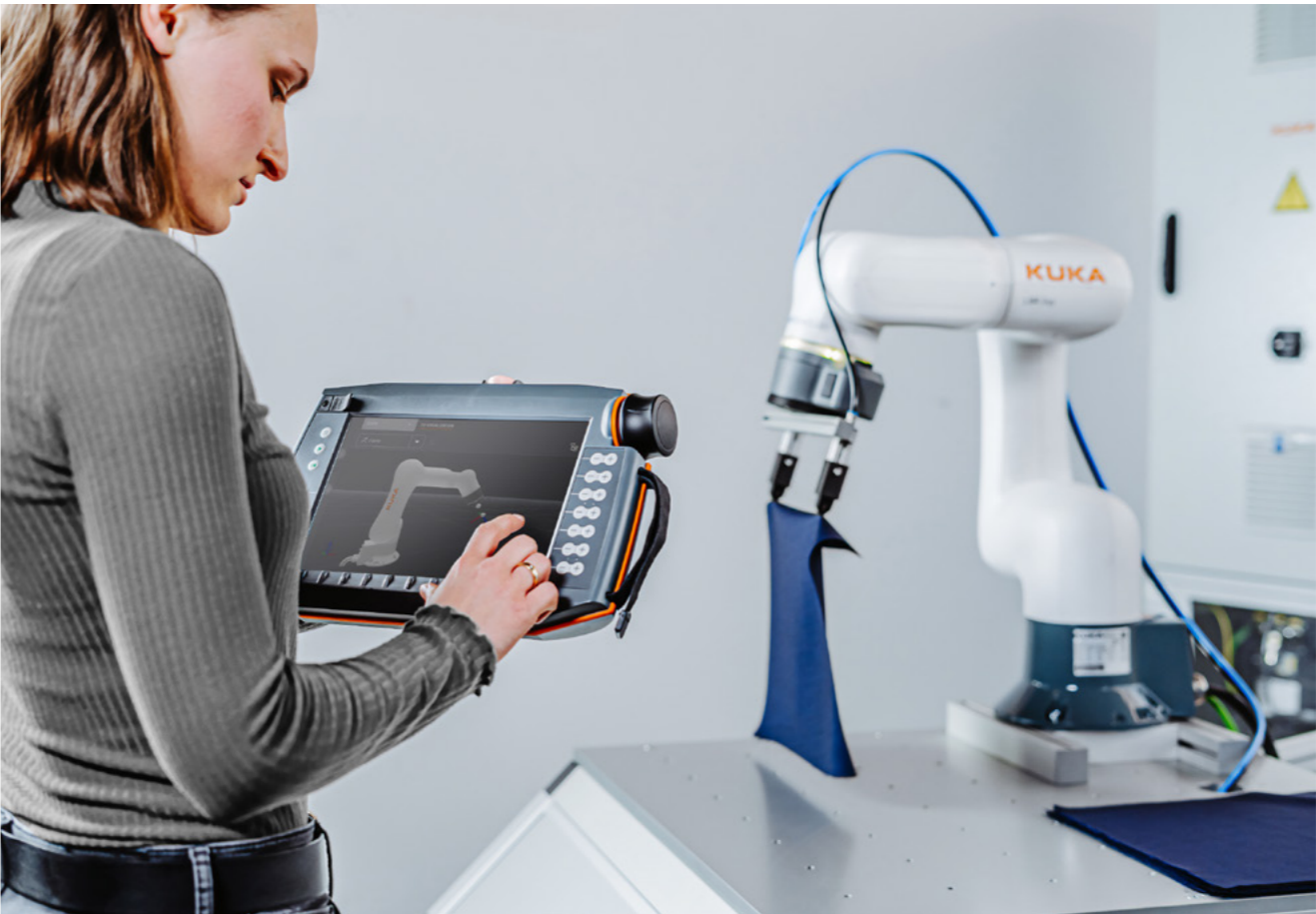
The handling of flexible, easily deformable, flexible textiles and cut parts, is possible with an LBR iisy robot.
