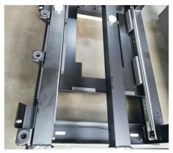
SNAPLOC® system, consisting of coupling and bolt, used in a seat of the company Probatec AG.
