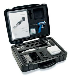
The new ONSERT® Portable allows manual processing. The joint between the workpiece and the ONSERT® fastener is created with a light-curing adhesive. The adhesive is manually applied to an ONSERT® fastener, then placed in the holder in front of the light source and held in position there by a magnet or mechanical means.
